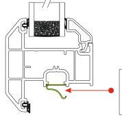
Fit a **BC002** Sash Spring to the sash on the center line of the stay fixing
